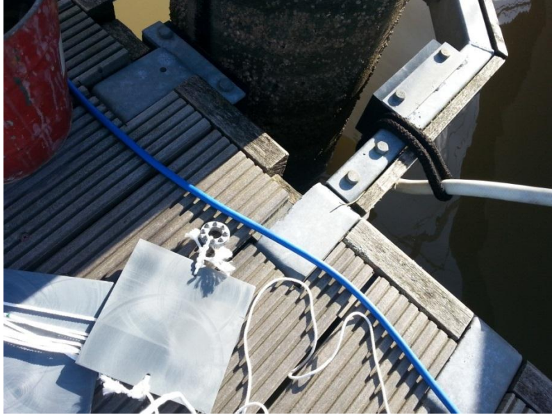
Figure 3.4 Vertical settlement panel with weight.
