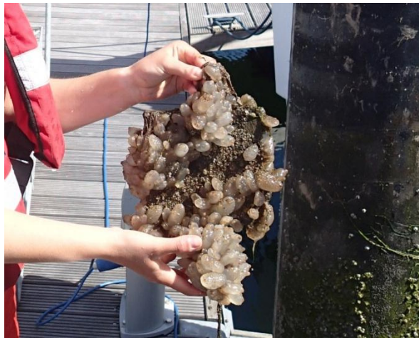
Figure 3.5 Vertical settlement panel collected on the 6 th July 2014 after 12 weeks of immersion in the visitor site at Milford Haven marina.
