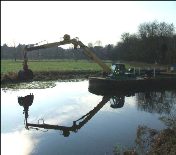
Mechanical excavation by barge can be used in faster flowing rivers,
