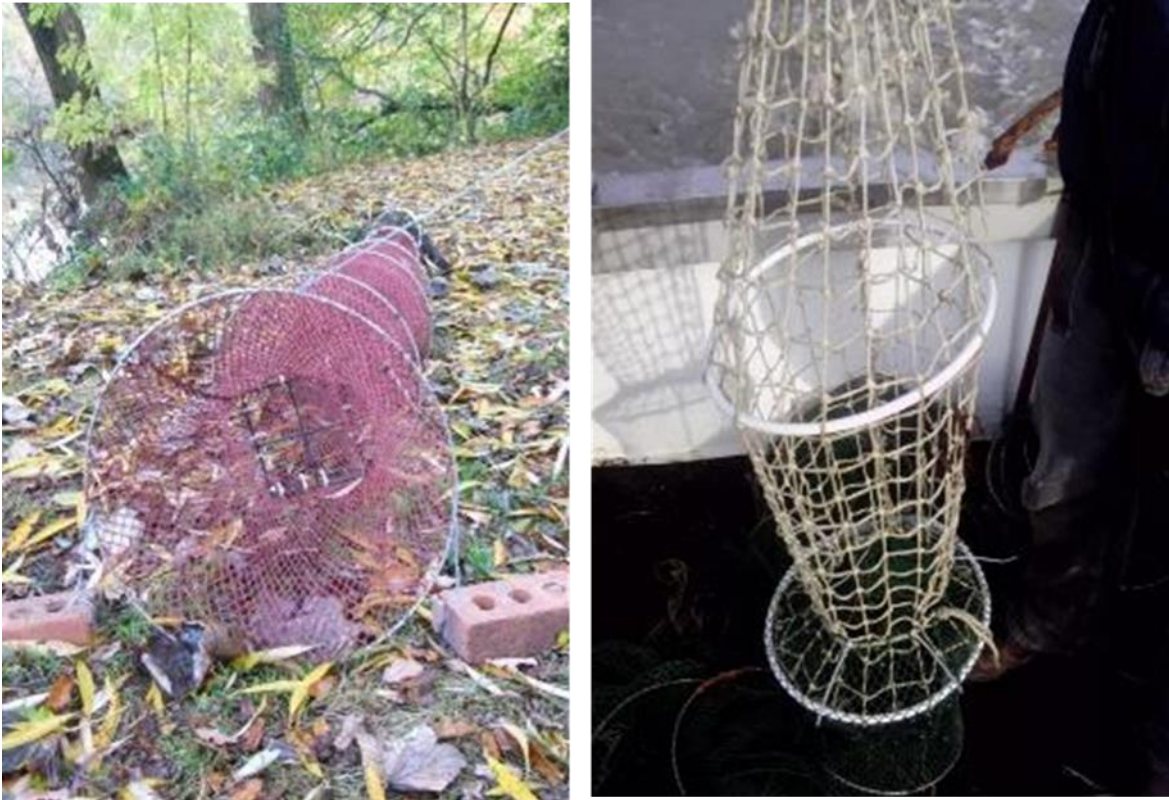
Figure 12. Fyke net without leaders as used in the 2013 trapping period. Otter guard visible attached in the entrance of the trap (left). 40mm mesh attached to end of fyke nets to reduce eel by-catch (right)
