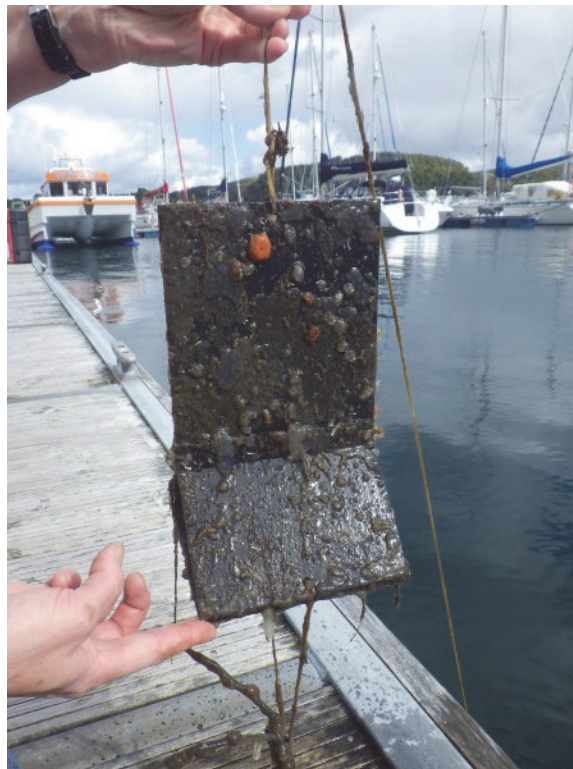
Figure 2. Settlement panel design used at all sampling locations. (Photo: C. Beveridge, SAMS).
