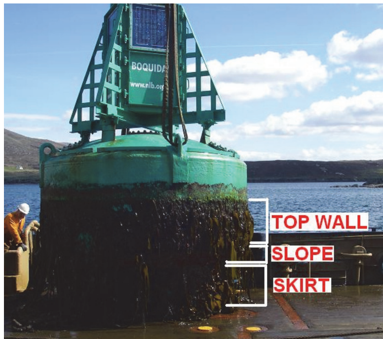
Figure 1: Showing the various parts of the buoy.
