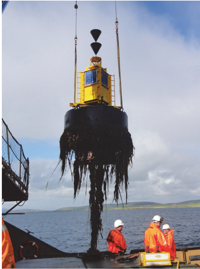
Figure 5. Retrieval of Northern Lighthouse Board navigation buoy for routine maintenance (Photo: A. Macleod, SAMS)
