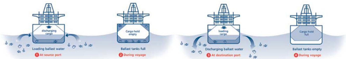
Figure 1: Transfer of non-native species due to ballast operations (from IMO, 2019 2 )
