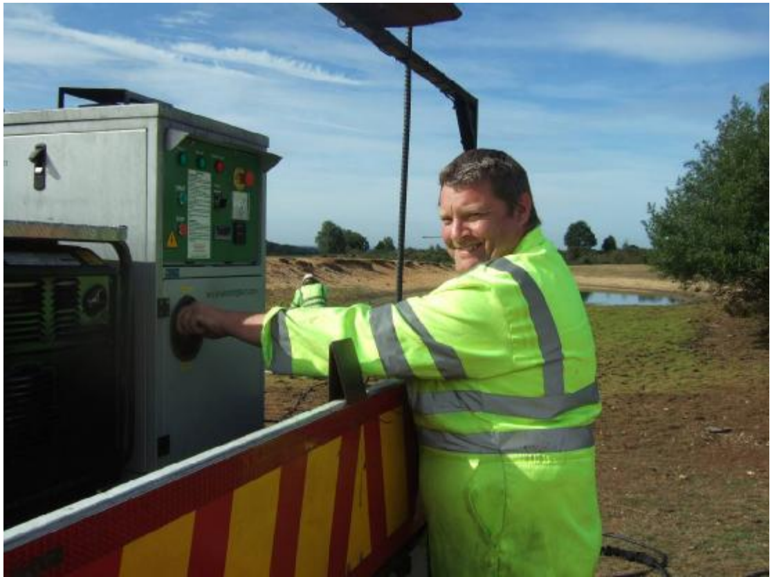
Anthony Clements adjusting the temperature controls on the equipment which is mounted on the 'amenity' vehicle.
